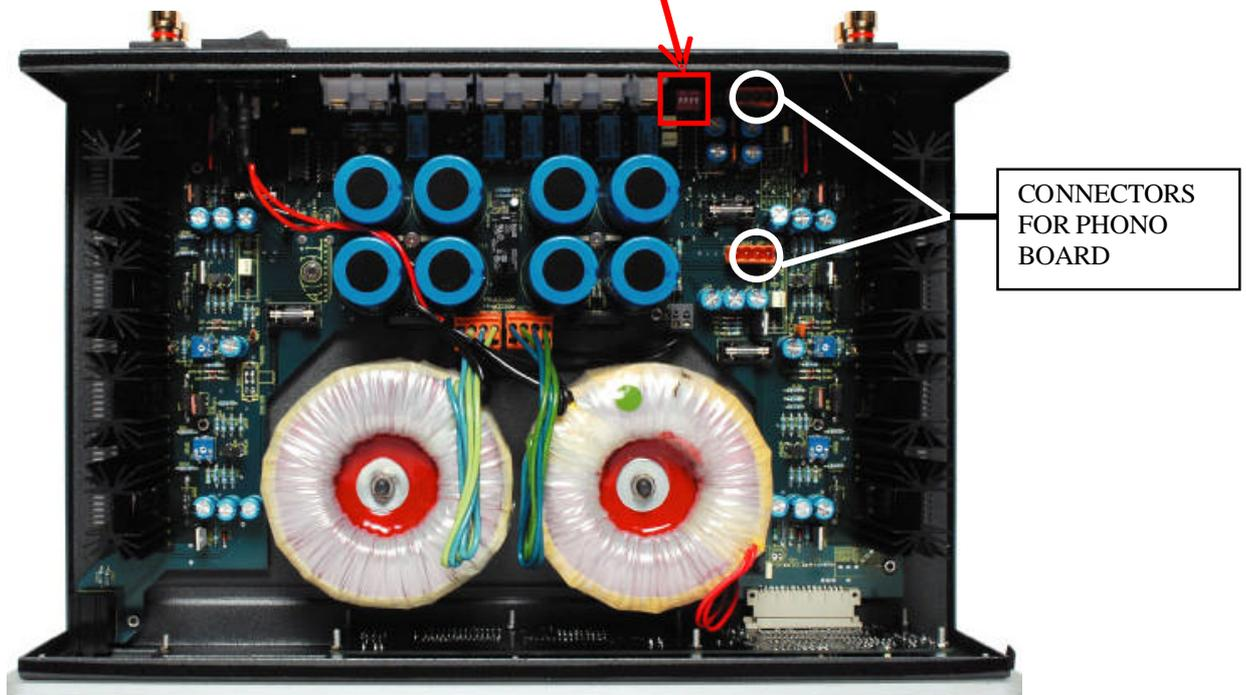
3- PLACE THE PHONO STAGE ON THE ORANGE CONNECTORS OF THE MAIN BOARD. (ONLY ONE WAY POSSIBLE)
